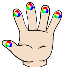
Figure 5. Placement of LEDs and RGB colour sensor
