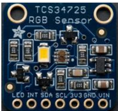
Figure 6. RGB colour sensor with IR filter
