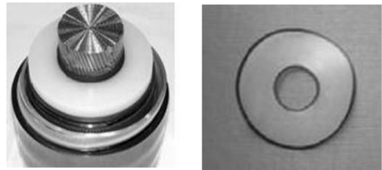
Fig. 1. Samples taken from a HV cable insulation.
