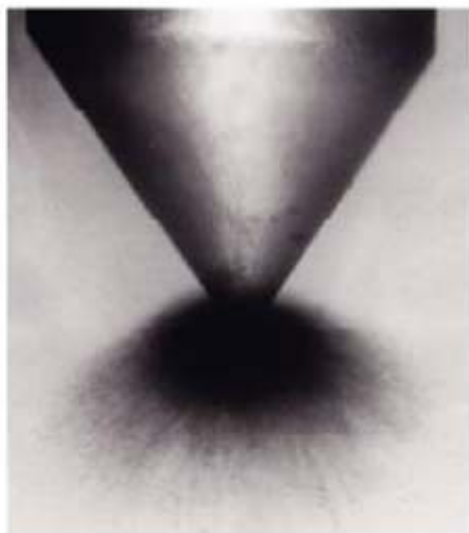
Fig. 1. Water trees in a low density polyethylene needle-plan sample: 1 – water needle; 2 – water trees ( U = 3 \text{ kV} , f = 13 \text{ kHz} , r_0 = 5 \text{ }\mu\text{m} , \tau = 250 \text{ h} ).
