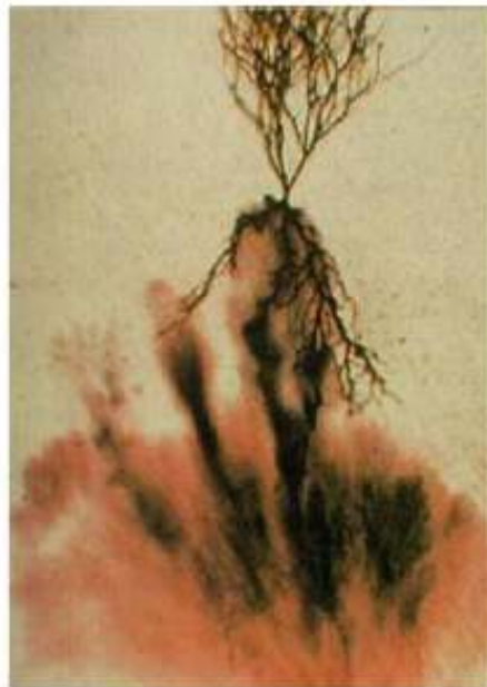
Fig. 4. Electrical tree inception in front of a water tree one.
