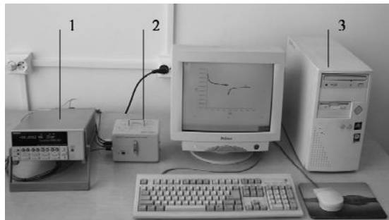
Fig. 3. Experimental set-up for absorption/resorption currents measurement: 1-Electrometer Keithley 6517, 2-Resistivity Test Fixture Keithley 8009, 3-PC.
