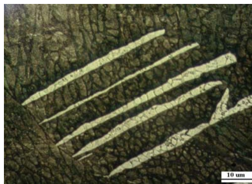
Imagini de microscopie optică aliaj SnBiSb; (a) x150, (b) x300; Atac chimic
