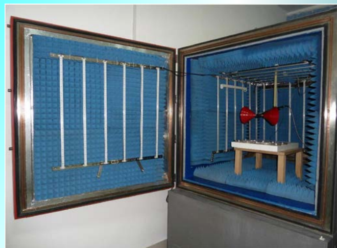
Fig. 5 Radio frequency electromagnetic field exposure system, [5]
