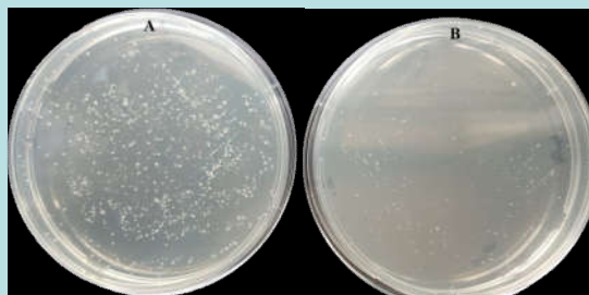
Fig. 7 Bacterial colonies formed on LB agar, inoculated with 10^4 dilution samples of activated sludge: A sample exposed to 60 mV/cm (50 Hz), B sample not exposed to ELF field.
