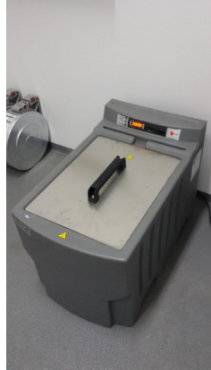
3D Printer for models Fortus 360 mc LE type made by STRATASYS - USA
