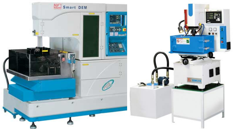
Processing Machines by electrical erosion: - with wire -left - with electrode -right
