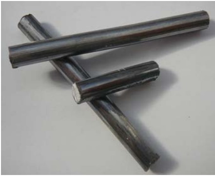
Extruded bars of Al-SiC composite material
