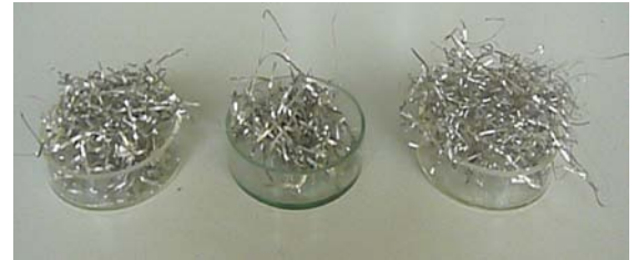
Amorphous metallic glasses: a) Fe-based amorphous sheets - copper mould casting, b) Fe-based amorphous strips - spin melting on copper rotating drum
