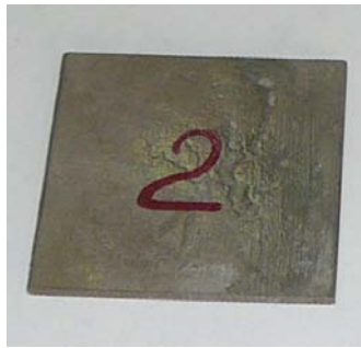
Amorphous metallic glasses: a) Fe-based amorphous sheets - copper mould casting, b) Fe-based amorphous strips - spin melting on copper rotating drum
