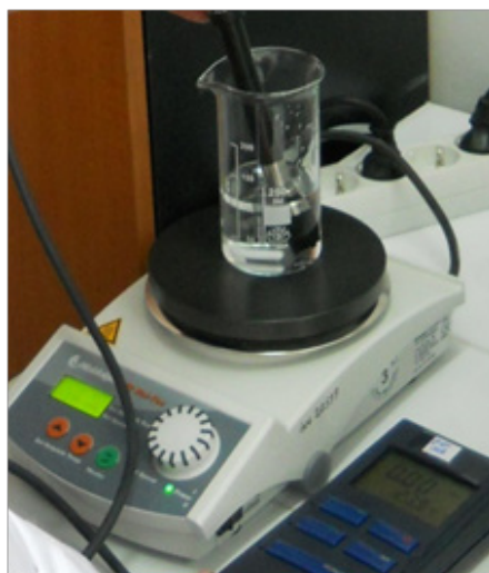
A Magnetic Stirrer Hotplate, HEIDOLPH type, MR Hei-Tec model
