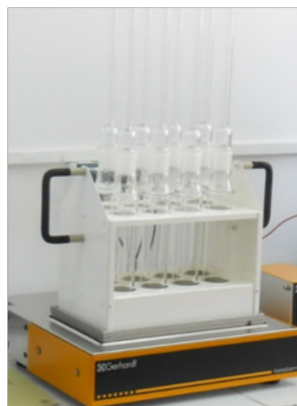
Chemical Oxygen Demand Analyzer GERHARDT type, Kjeldatherm model
