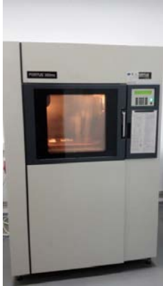
3D Printer for models Fortus 360 mc LE type made by STRATASYS - USA
