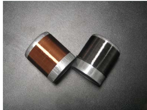
Different spools with microwires from FeBSi and copper
