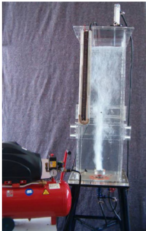
Equipment for determining the hydro-gas-dynamic performances of fine bubble generators
