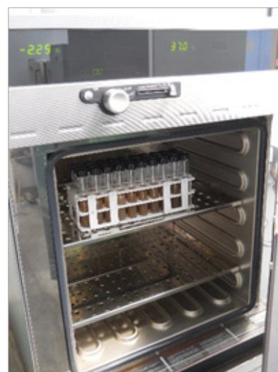
Oven/Incubator/Sterilizer, Mettmert type
