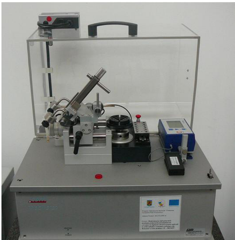
Equipment for tribological characterization of the thin films
