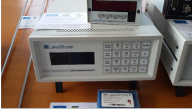
Temperature Monitor 218 type
