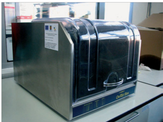
BOD Thermostatic Box, WTW type, OxiTop Box model
