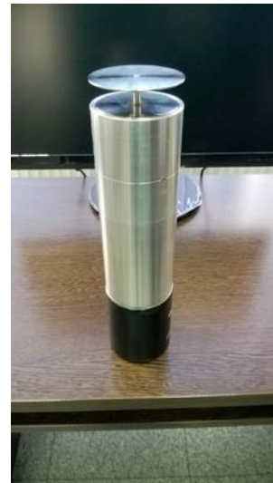
Linear magnetostrictive motor for outer space applications
