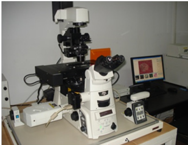
Inversed Optical Microscope, Nikon Eclipse Ti-E type, fitted with confocal system Eclipse C1si
