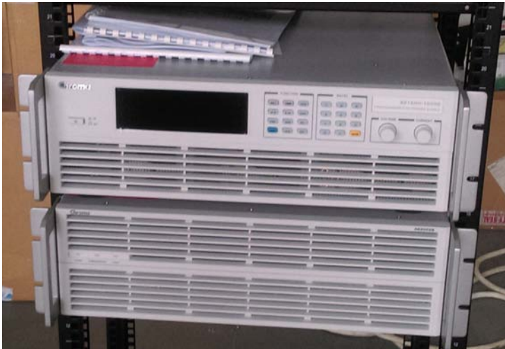
62150H-600S/1000S model 600V/1000V/15kW
