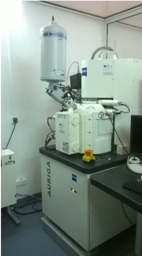
Scanning Electron Microscope (FESEM-FIB) Auriga Zeiss type
