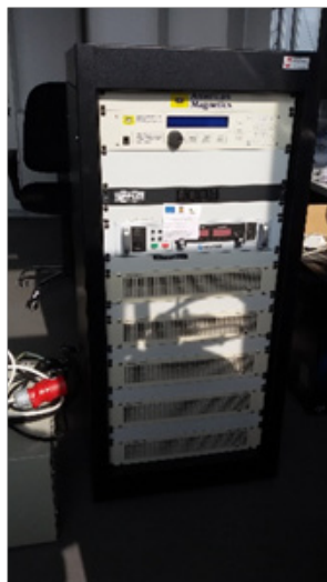
Programmable DC power supply XR10-600/208 type
