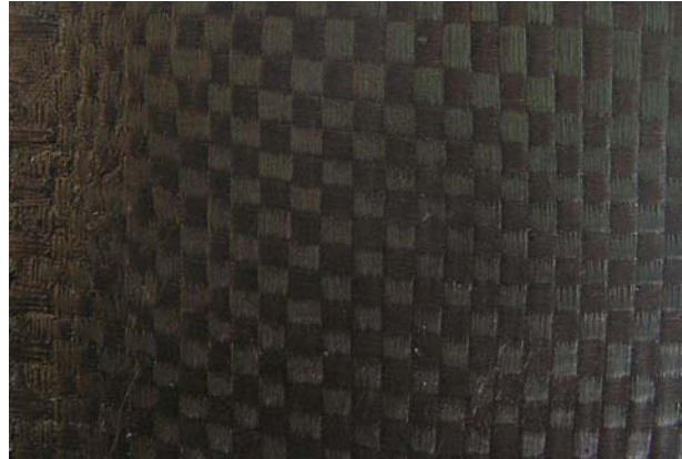
FC composite impregnated with epoxy resin reinforced with carbon nanotubes
