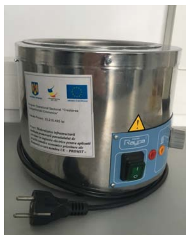
Thermostatic Water Bath RAYPA type, BAC-1 model
