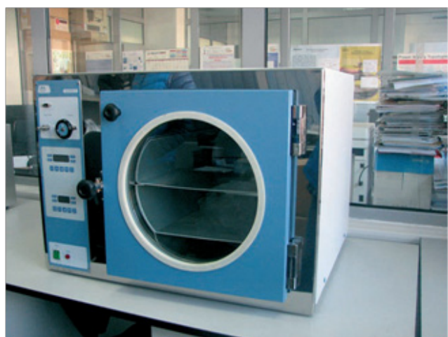
Vacuum Drying Oven SELECTA type, Vaciotem-T model
