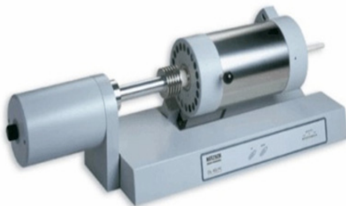
Dilatometer DIL 402 PC/4, made by NETZSCH Gerätebau GmbH - Germany
