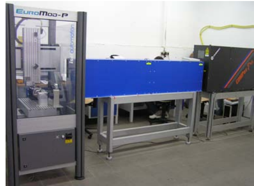
Excimer processing laser station (KrF) of Coherent COMPex Pro 205 F type
