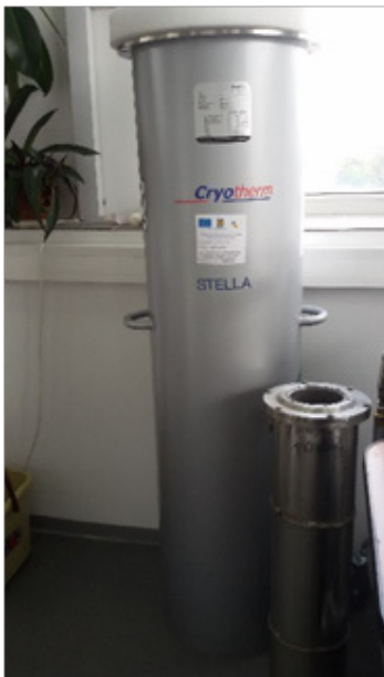
Cryostat for the liquid nitrogen STELLA F 300/1250 type
