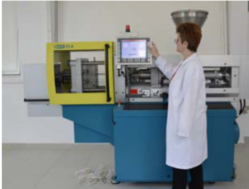
Melt Injection Machine BOY 35A type
