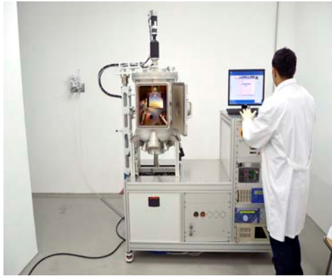
Technological Equipment for Vacuum Processing of Titanium Nitride Thin Layers ETPV-SSNT type made by BESTEC Germany
