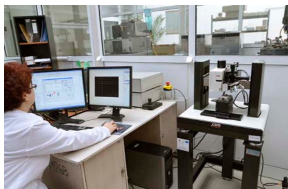
Equipment for tribological characterization of the thin films
