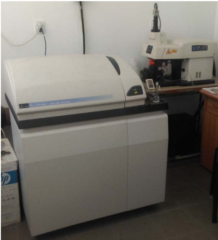
Laser Ablation Mass Spectrometer ELAN DRC type
