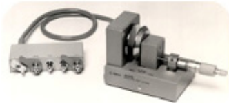
Dielectric Measuring Kit 16451B, 40 Hz to 30 MHz
