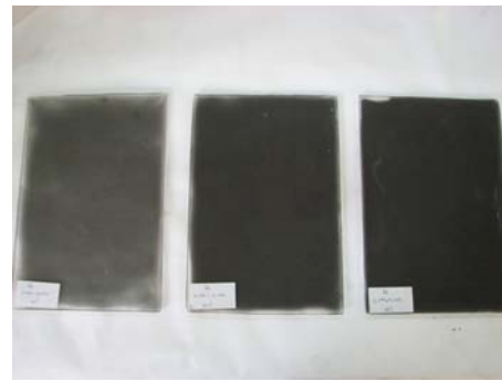
Electromagnetic shields with Fe grain size of 0.040 - 0.050 \mu\text{m} , 0.050 - 0.080 \mu\text{m} at concentration of 4%, 10%, 16%
