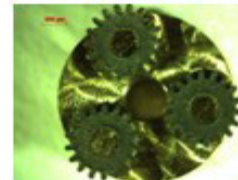
Port-satellites for planetary microreducer, 3.4 mm, optical microscope x 25
