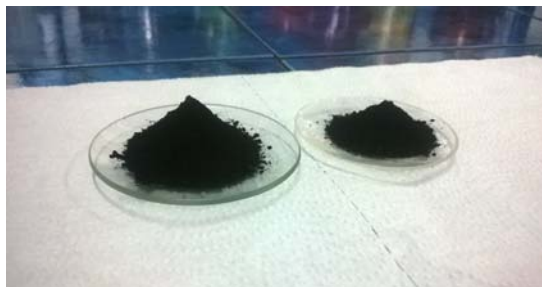
\text{FeNi}_3/\text{Al}_2\text{O}_3 and \text{FeCo}/\text{Al}_2\text{O}_3 core-shell nanopowders
