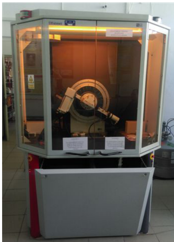
X-ray Diffractometer D8 ADVANCE type
