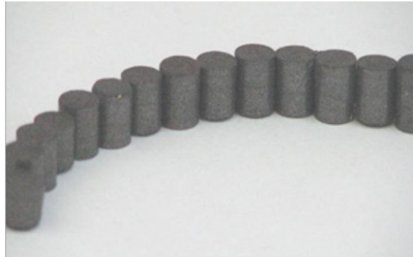
Magnetic and physical properties of NdFeB bonded permanent magnets
