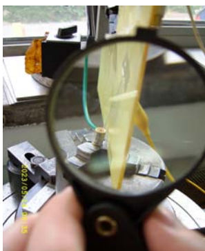
Fixing on transducer dividing head and fixing the measuring connections
