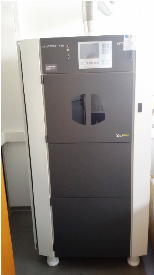
Equipment for exposure to light and climatic aging XENOTEST 440 type made by ATLAS - Germany
