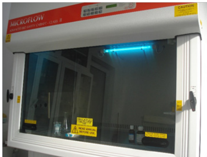
Biological Cabinet Astec Microflow, ABS 1000 model
