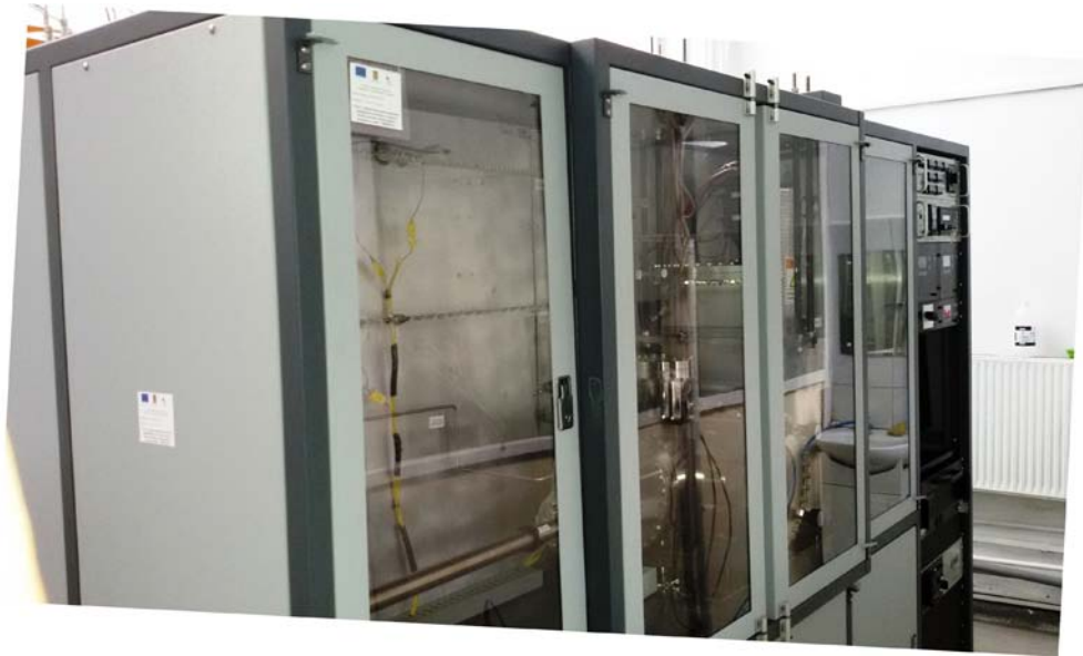
Plasma-Enhanced Chemical Vapor Deposition (PECVD) for flexible organics
