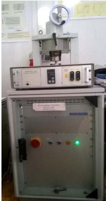
Hysterezisgraph type AC/DC Hystograph - Brockhaus Messtechnik -
