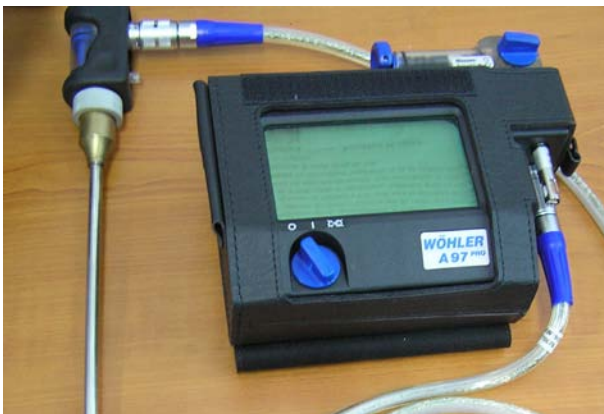
Emission Gas Analyzer A97PRO type, made by WTW GmbH
