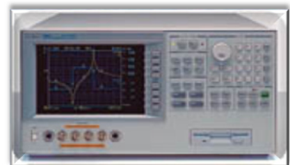
Impedance Analyser 4294A Measurement range: 40 Hz - 110 MHz
