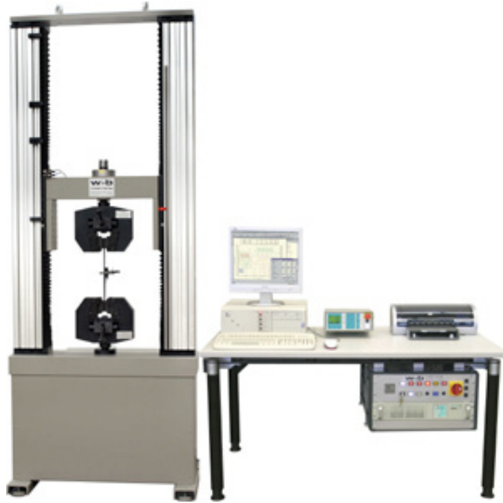
Static Universal Testing Machine for Materials LFM 30kN type, Walter & Sai AG Switzerland
