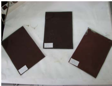
Electromagnetic shields with Cu concentration of 4%, 8%, 16%
