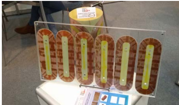
Assembly coil with cylindrical shape for particle accelerators
