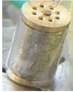
Prototype of non-contact angle transducer (increase with magnifying glass)
