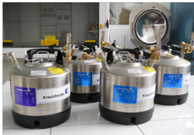
Pressure vessels for 0, 2, 4, 6 bar, KRAUTZYBERGER type
