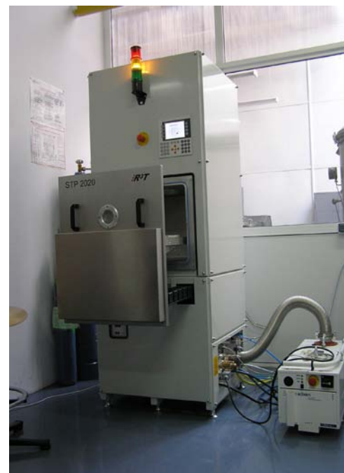
Remote Microwave Plasma Etcher STP 2020 Stripping Tool for SU8, made by R3T - Germany
