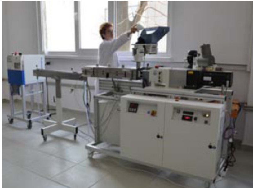
Plastic Materials Laboratory Extruder KETSE 20/40 type
