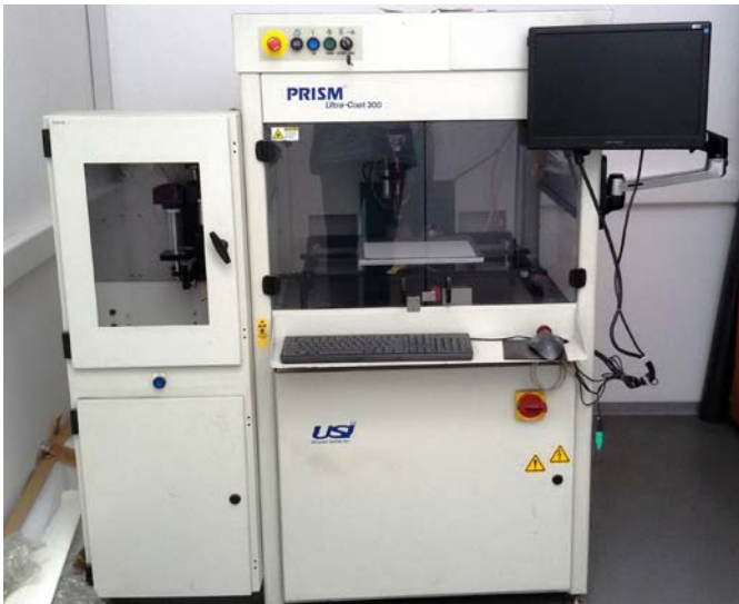
Automated system for the thin layers depositon by "SPRAY" technique PRISM Ultra-Coat 300 type made by Ultrasonic Systems Inc. - USA
