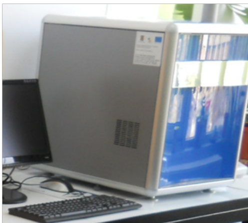
Total Organic Carbon/Total Nitrogen (TOC/TN) Analyzer, ELEMENTAR type, VarioTOC CUBE model
