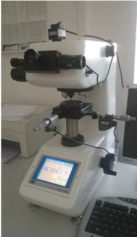
Microhardness Tester FM 700 type
