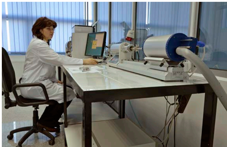
High Temperature and Resolution Dilatometer for Metallic Alloys L75HS2000C + L75HS700LT type
