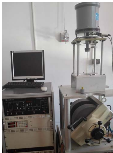
Vibrating Sample Magnetometer (VSM)
