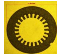
Sheet for electric microgenerator, optical microscope x 20, D=11mm
