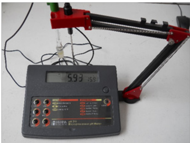
pH-meter, Hanna Instruments type, PH 211 model
