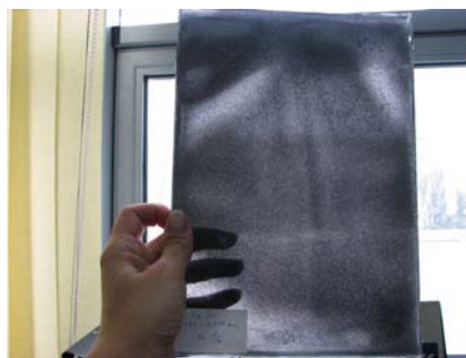
Electromagnetic shields with FeSi grain size of 0.040 - 0.050 \mu\text{m} at concentration of 10%
