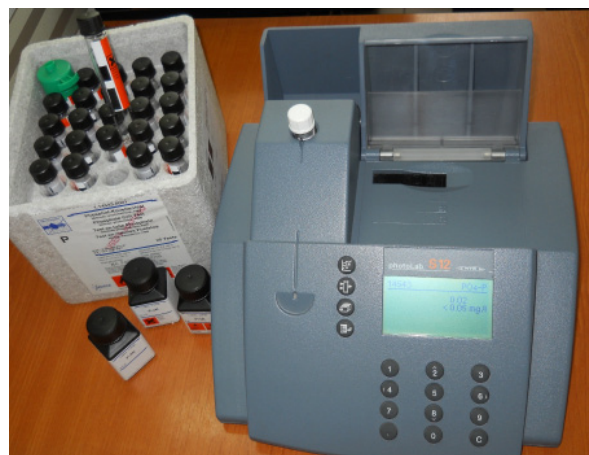
Spectrophotometer WTW Photolab S12 type
