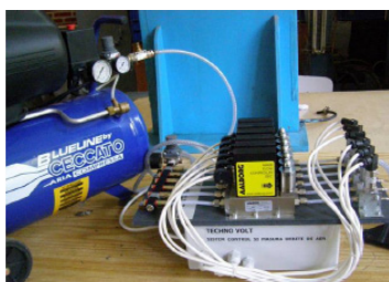
System for data acquisition, monitoring and control of pressures and flow rates on 6 channels
