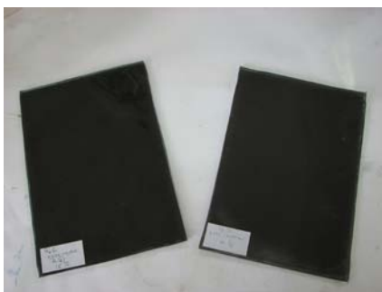
Electromagnetic shields with FeSi grain size of 0.036 - 0.040 \mu\text{m} , 0.040 - 0.050 \mu\text{m} at concentration of 10%, 16%
