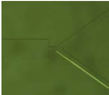
Microfluidic channels in SU8, optical microscope x 50
