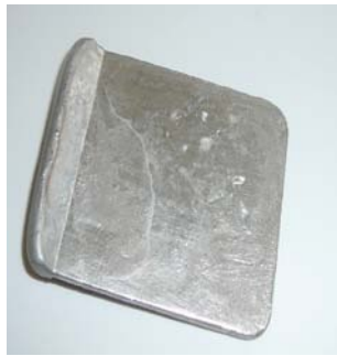
Amorphous metallic glasses: a) Fe-based amorphous sheets - copper mould casting, b) Fe-based amorphous strips - spin melting on copper rotating drum
