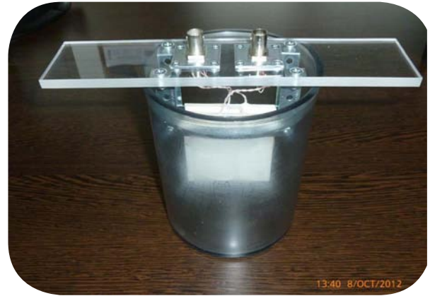
Transducer for measuring the dynamic viscosity in continuous flow using active piezoceramic elements
