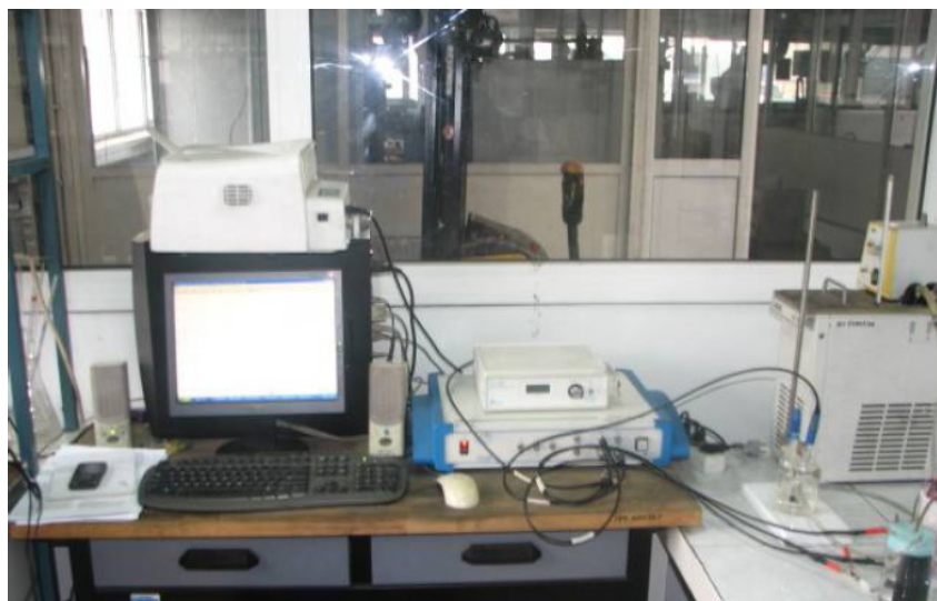
"All-in-one" potentiostat / galvanostat VoltaLab 40 Radiometer Analytical
