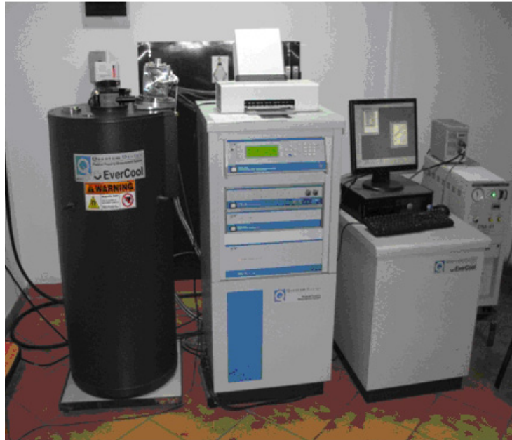
Measurement system of physical properties at low temperature, in range 4.2 ... 350 K
