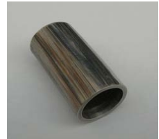
Extruded pipes of Al_2O_3
