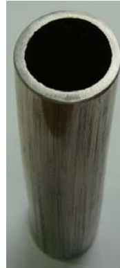
Extruded pipes of Al_2O_3
