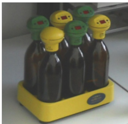
Biochemical Oxygen Demand Analyzer, WTW OxiTop - IS 6 type
