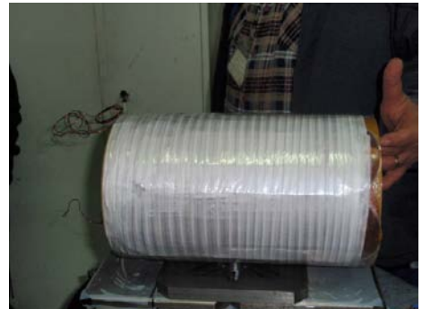
Assembly coil with cylindrical shape for particle accelerators
