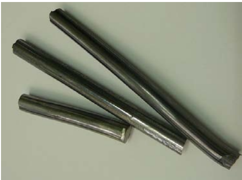
Extruded bars of Al- Al_2O_3
