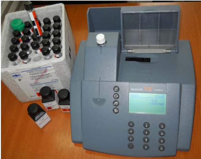
Portable Spectrophotometer WTW PHOTOLAB S 12 type
