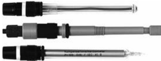
Fig.1: Cative senzori de ape, lungime ~150 - 200 mm; Ø ~ 12 mm (sursa JUMO / Germany)
