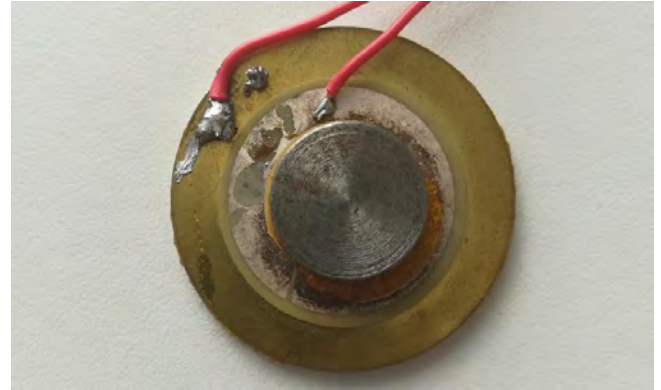
Fig. 7. The first generation experimental model accelerometer on an elastic membrane structure
