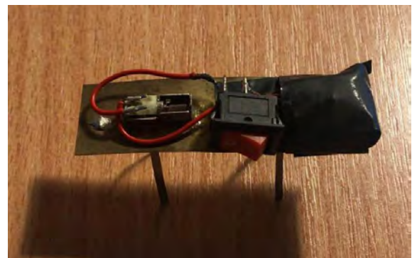
Fig. 11. Movement mechanism that replicates the locomotion of a real insect functioning with a switch
