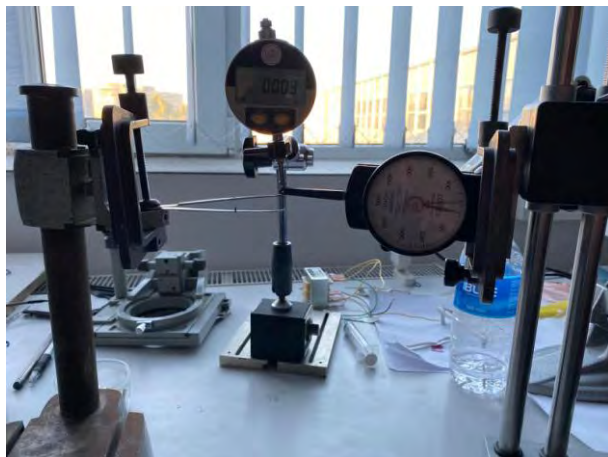
Fig. 5. Measuring the force needed to open a tweezers
