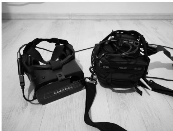
Figure 12: Helmet's Profile, HDMI Capture Chip Visible
