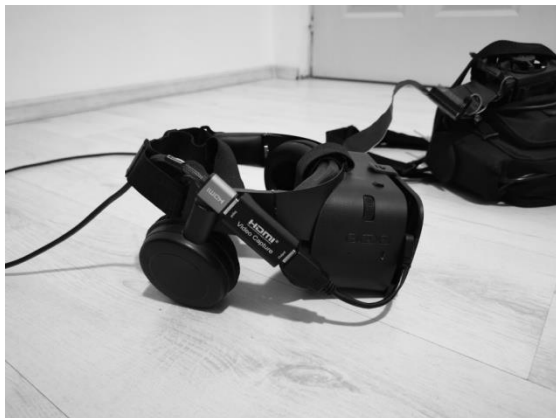
Figure 12: Helmet's Profile, HDMI Capture Chip Visible
