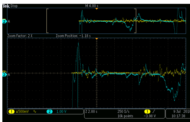
Fig. 3. The mechanical tension felt by the tissue (blue line) and the mechanical tension felt by the scalpel (yellow line)
