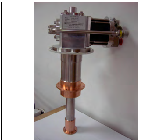
Fig. 2.18. Crioracitor cu doua trepte de racire – SHI Cryogenics.
