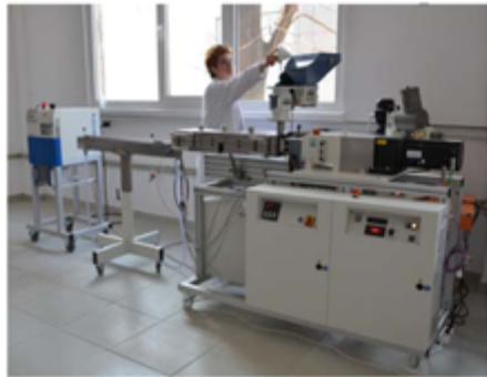
Extruder de laborator tip KETSE 20/40
