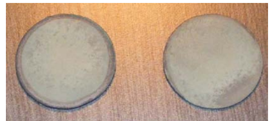
Samples of \text{Si}_3\text{N}_4 + \text{SiC} sintered at SPS
