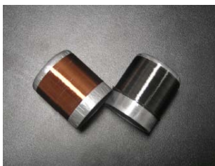
Spools with glass-coated microwires made from copper and Fe-Si-B alloys
