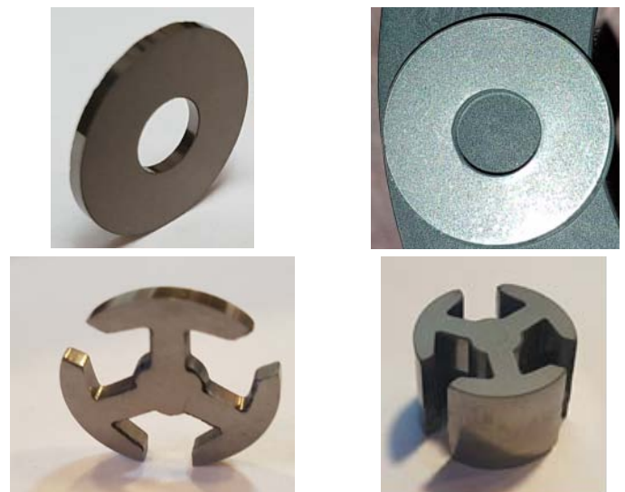
Rings, rotor core and 4 rotor cores stack, made from FeCo electrically insulated nanopowders
