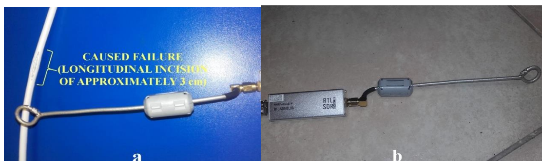
Fig. 3. Cable caused failure (a) and the complete tool prepared for evaluation (b).
