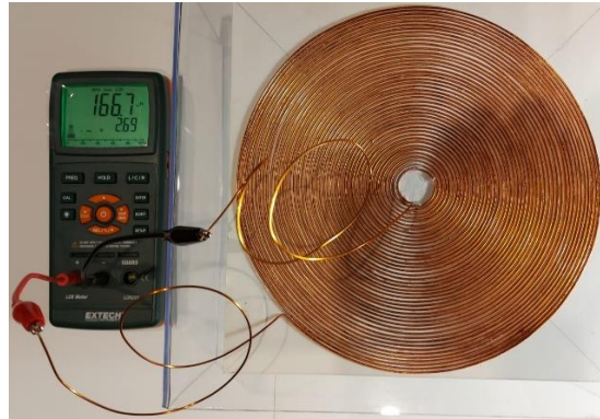
Fig. 2. Planar spiral coil self inductance real measurements
