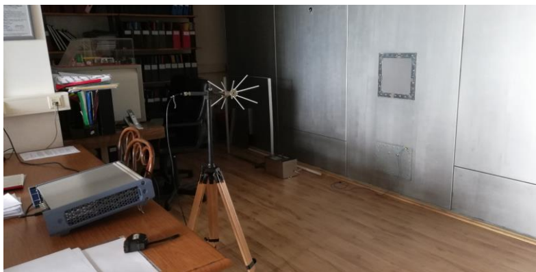
Fig. 2. The location used to measure the shielding performance of the material
