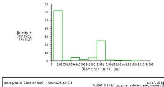
Fig. 1.2, The distribution of Sauter diameter for the classes of bubbles from tank
