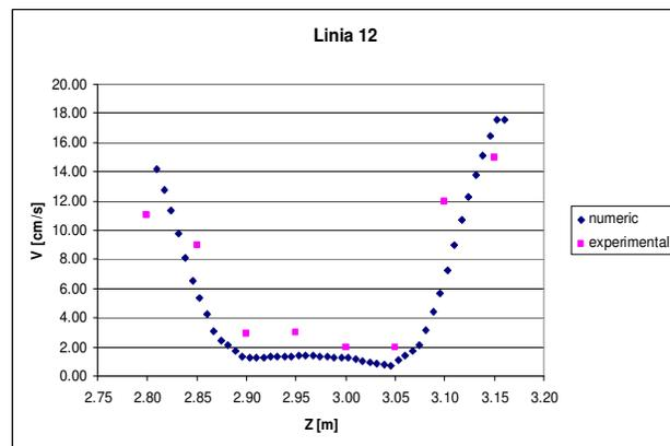
Fig. 5.2, Induced velocity variation at a distance of 40 cm from the diffuser, at the middle of the distance between 2 lines with porous diffusers.
