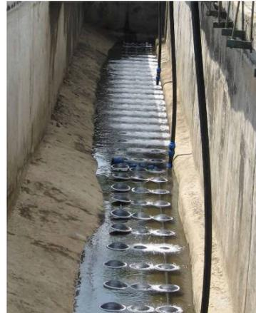
Fig. 2.4, Installation for determining the mass transfer in situ
