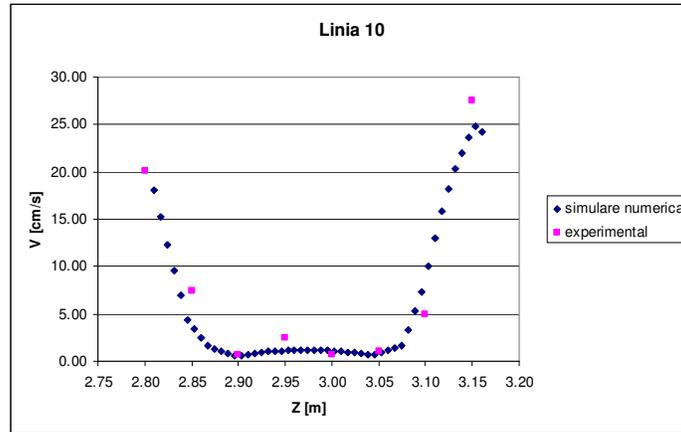
Fig. 4.1, The variation of the velocity  $V$  in function of the coordinate  $Z$ , at a distance  $X=20$  cm from PD
