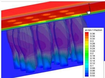
Fig.1.1, The density of the class of bubbles with diameter  $d = 0.0019$  m
