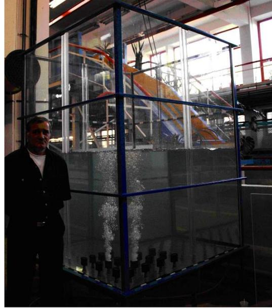
Fig. 2.2, Installation for testing a network of PD  $\Phi 50$
