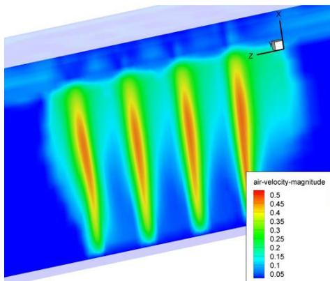
Fig. 5.1, Air velocity field for porous diffusers at  $y = 0,295$  m
