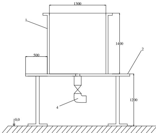
Fig. 3.2, Open channel – front view (1- tank, 2 – deck, 3 - fose Φ2'')
