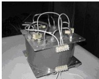
Fig. 1 Heating system with quartz lamps
